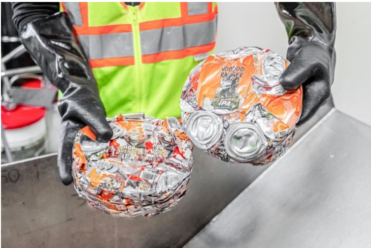
Picture 5: The compressed discs are 200 mm in diameter.
