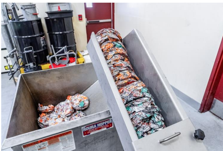
Picture 3: Compressed discs are discharged via a discharge pipe
