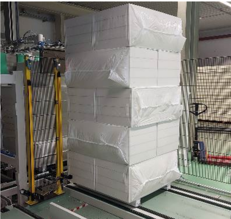
Bundles of PUR panels in new 6-sided packaging. Uniform packaging by use of a stretch hood film, with sealing in each for full sealing.
