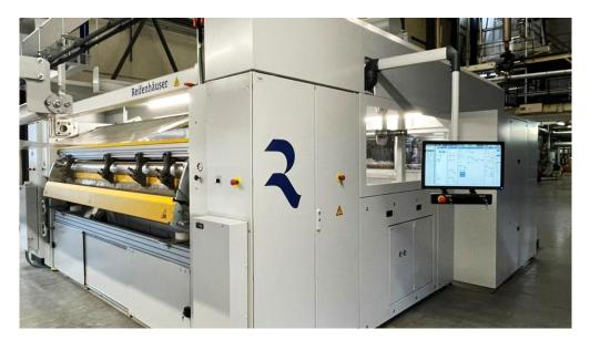
PAM can be conveniently operated via the system HMI. Once recipes have been saved, they can be reproduced at the touch of a button, even by less experienced system operators.
