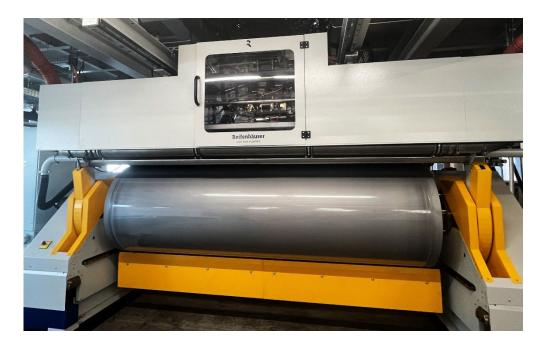
The die and feedblock automation works completely autonomously and contact-free in an enclosure. In addition to easy operation, the system also offers maximum work safety.
